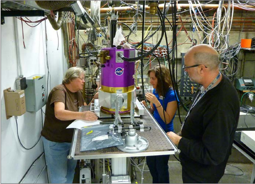
Figure 8-7. NEOCam detector development. The cylindrical object in the center is a cryogenic chamber used for cooling the detectors. Left to right, Judy Pipher of the University of Rochester, Amy Mainzer of the University of Arizona, and Mark McKelvey of NASA Ames Research Center. (Image courtesy of Amy Mainzer)
