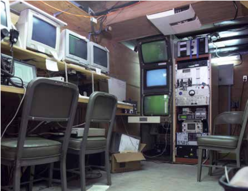
The Perseus GCS included positions for a pilot and several systems monitors. NASA
