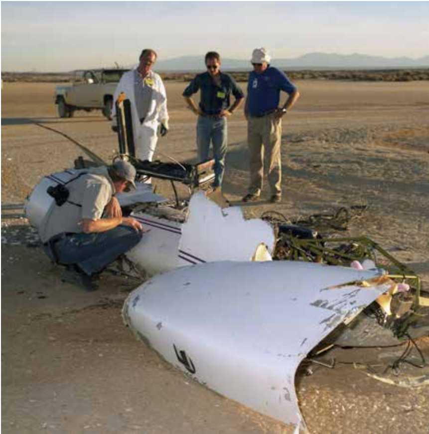
Investigators examine Theseus wreckage at the crash site near the north end of Rogers Dry Lake, within the boundaries of Edwards Air Force Base. NASA
