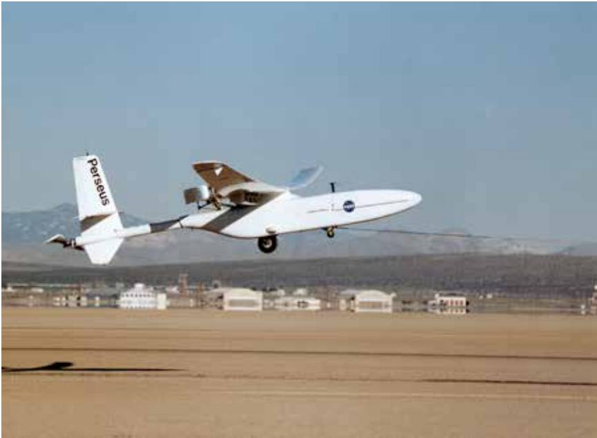
The second Perseus-A vehicle, AU-003, is towed aloft from Rogers Dry Lake at Edwards Air Force Base. NASA
