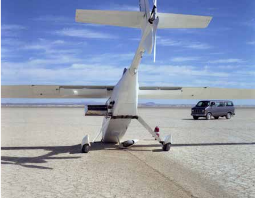
Nose-gear collapse following the maiden flight of Perseus-B damaged the vehicle's composite nose assembly. NASA
