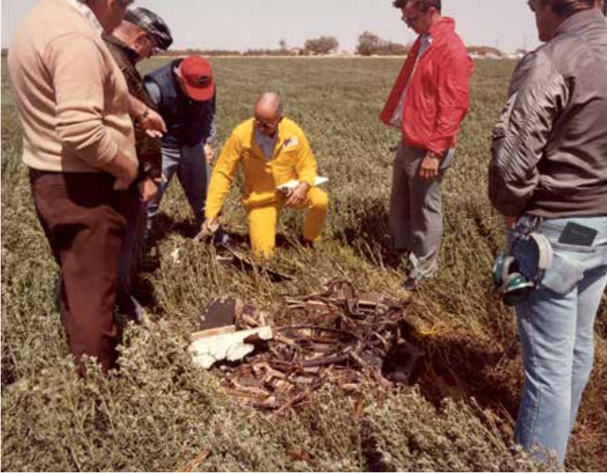
Investigators examine the DAST-2 wreckage at the crash site. The primary cause was traced to an electrical problem. NASA
