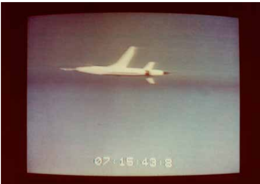
With only one remaining wing, the DAST-1 plummeted toward the ground. NASA
