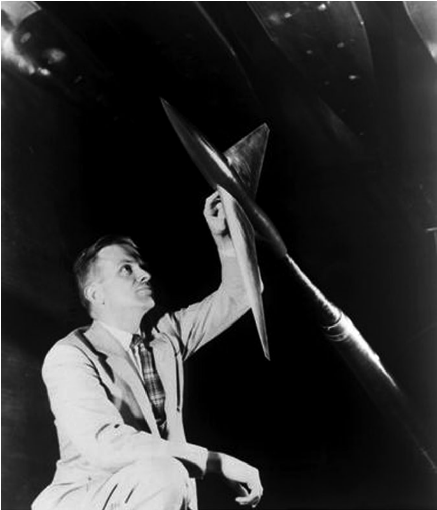
Richard T. Whitcomb examines a model incorporating his famous transonic area rule in the 8-foot High-Speed Tunnel in April 1954. (NASA Langley Research Center [NASA LaRC].)
