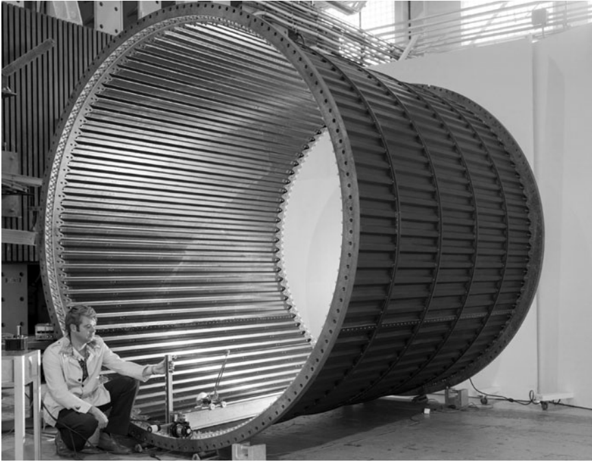
The corrugated shell is made from thermoplastic composite materials (February 17, 1978). (NASA Langley Research Center [NASA LaRC].)
