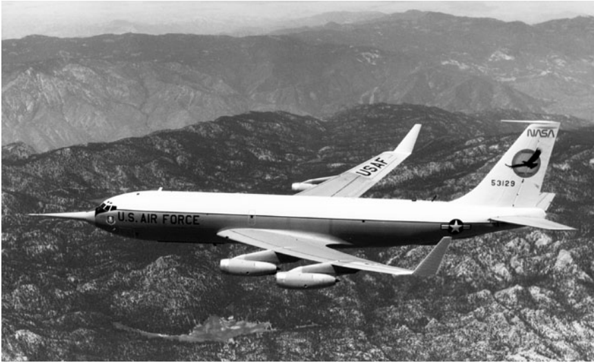
A KC-135 with winglets in flight over the San Gabriel Mountains, south of Edwards. (January 1, 1979). (NASA Dryden Flight Research Center [NASA DFRC] Photo Collection.)
