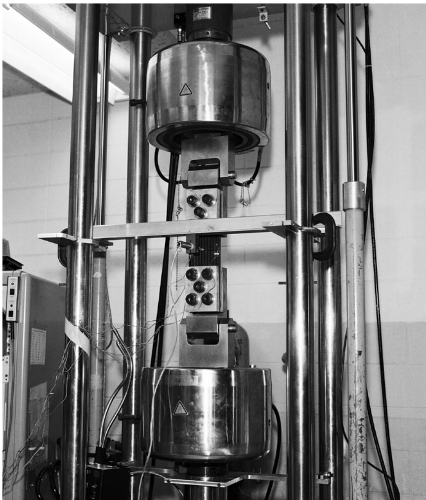
Advanced Subsonic Technology test apparatus for combined bending and membrane test at Langley (November 7, 1997). (NASA Langley Research Center [NASA LaRC].)
