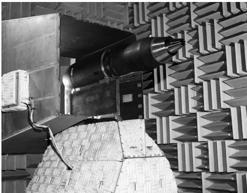
Bypass ratio 5 separate flow nozzle with chevron noise suppression trailing edge, photographed at Langley (October 20, 1999). (NASA Langley Research Center [NASA LaRC].)
