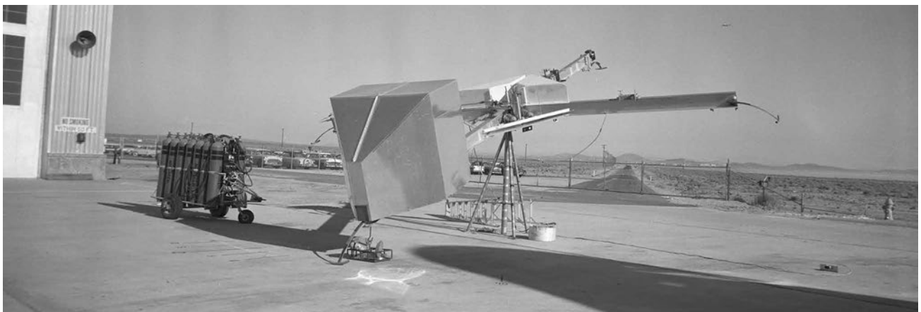
The final configuration of the Iron Cross, showing the full enclosure for the pilot and the bottles of compressed nitrogen for thrust. E58-3669.
