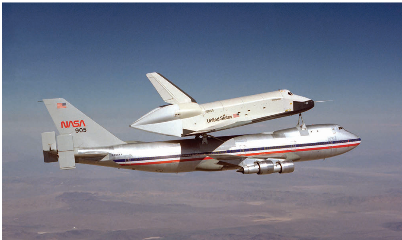
Enterprise mated to the SCA conducting captive-carry flights at Edwards AFB. NASA ECN-6887
