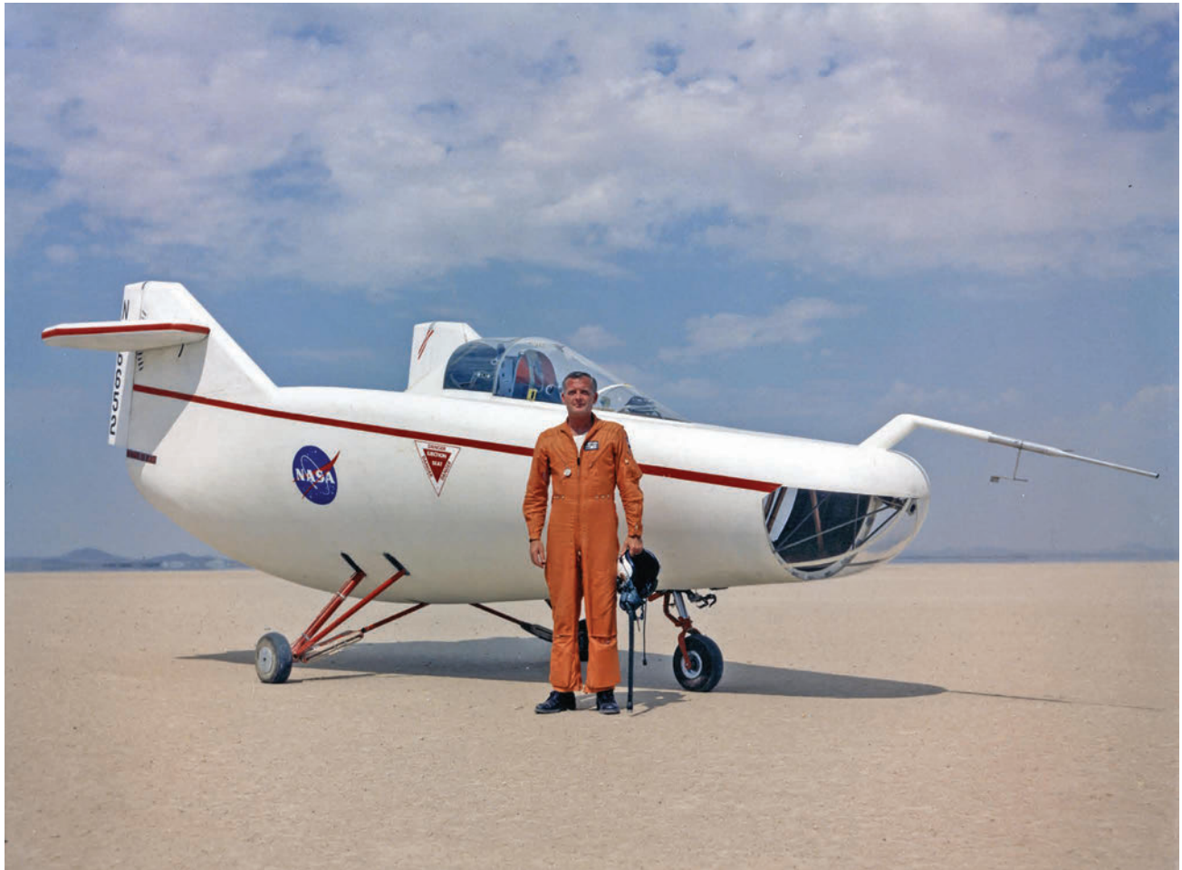
Milton O “Milt” Thompson standing next to the M2-F1, the world’s first full-scale lifting body, which he was the first to fly. NASA EC62-206
