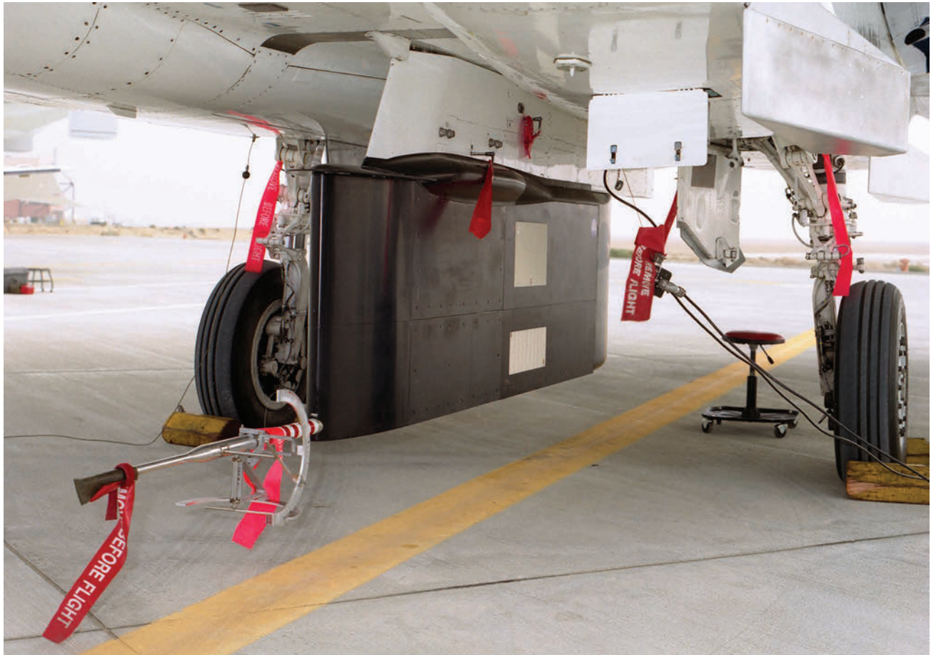
The Aircraft Flight Test Fixture attached beneath Dryden's F-15B. On the right side are two pieces of External Tank foam embedded in the test fixture; they are light in color compared to the rest of the fixture. NASA EC05-0030-01
