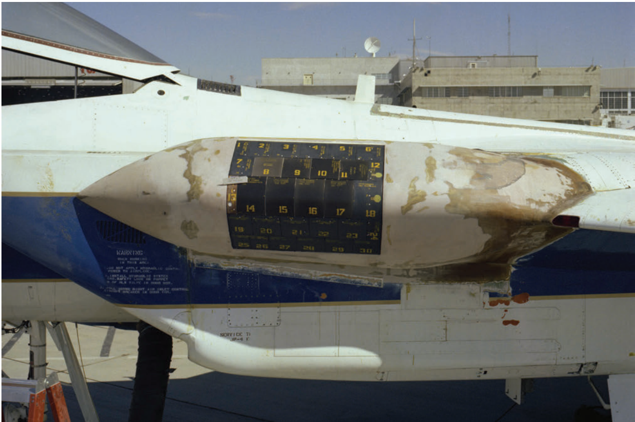
The leading edge of the F-15B sporting pieces of the shuttle tile. NASA EC80-13386
