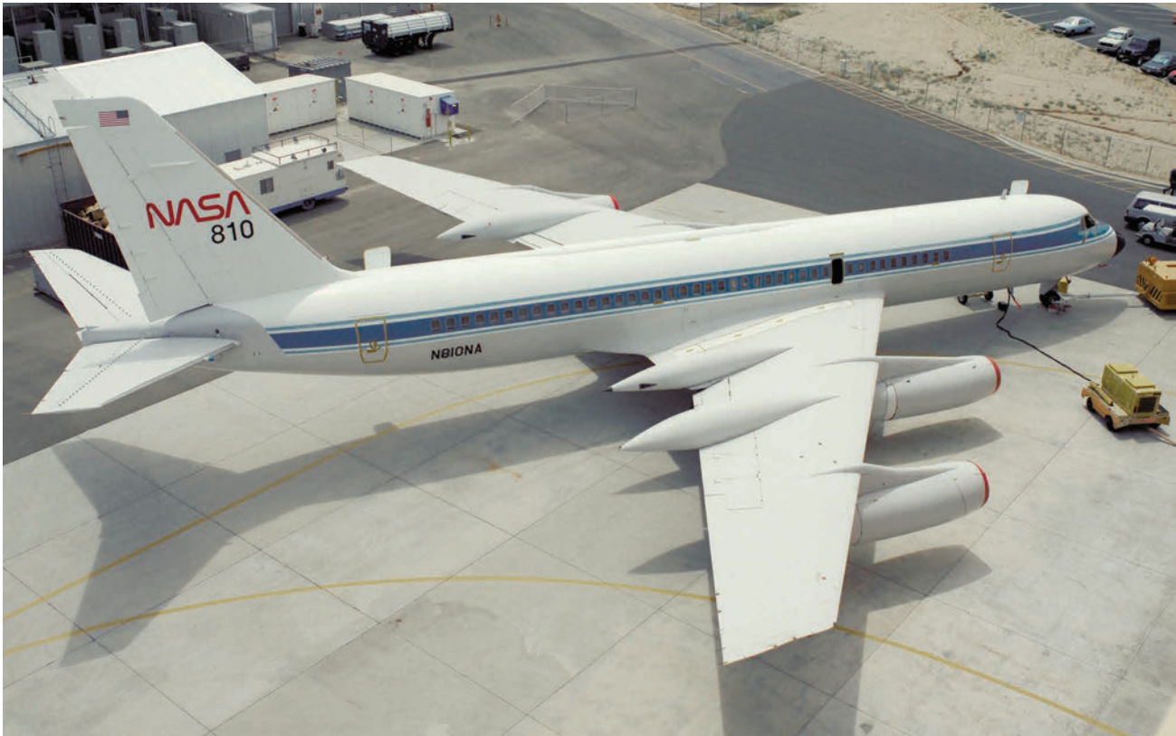
The CV-990 LSRA at Dryden. This angle highlights the aerodynamic shock pods on the wing’s trailing edge necessary to reduce drag and allow the aircraft to reach its maximum operating speed. NASA EC92-057275-30
