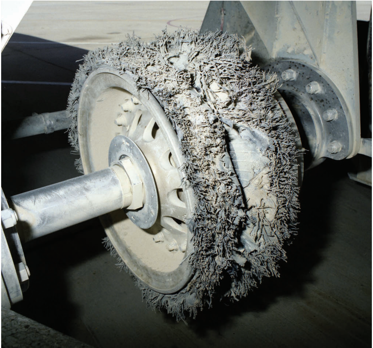
This tire, tested to destruction at Dryden, looks similar to ones subjected to the CV-990 first landings one KSC's runway during Round 1 of testing. EC95-43229-01
