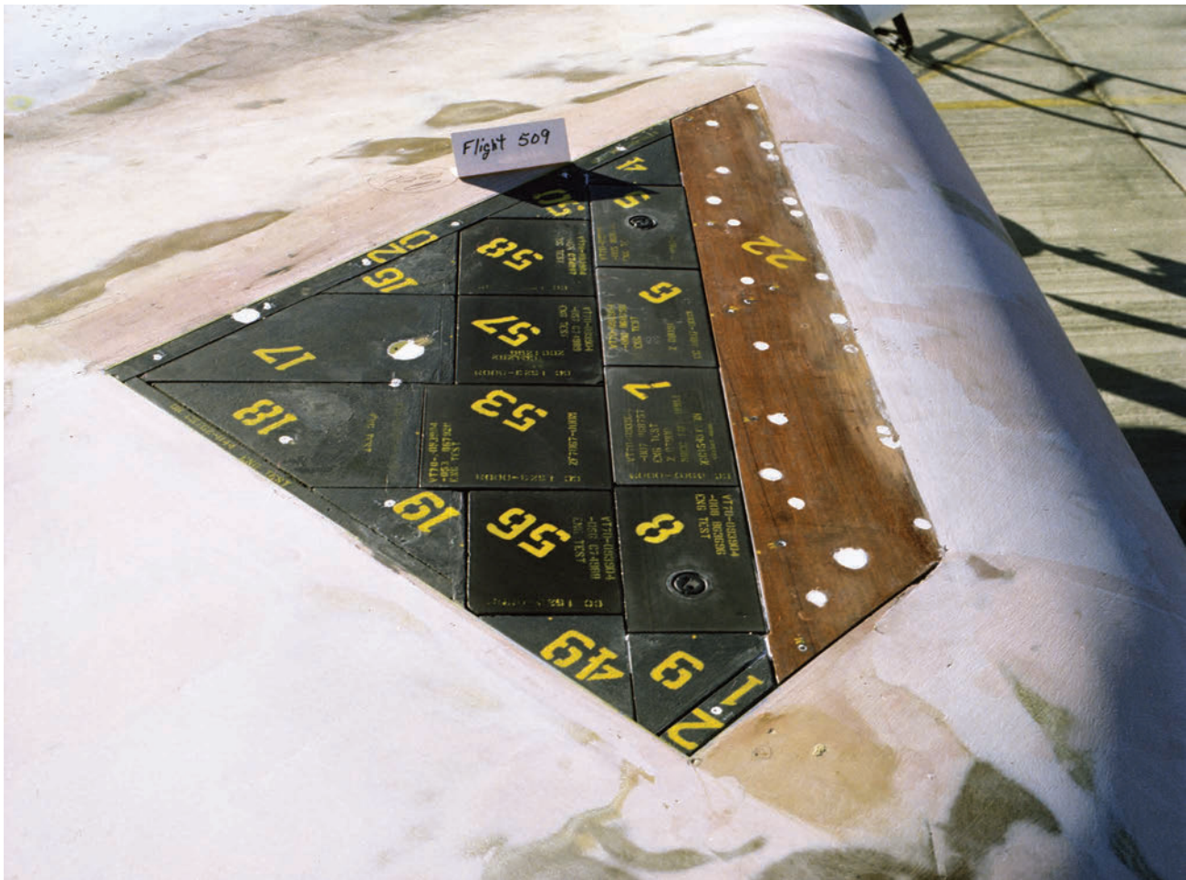
The F-15B's right wing layered with shuttle tiles for flight. NASA EC80-12253
