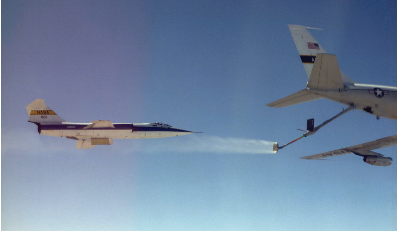
The F-104 in flight behind the Air Force icing tanker spraying water. The tanker was designed to test anti-icing systems on Air Force aircraft and NASA initially used it to test the Thermal Protection System tiles for the shuttle. NASA EC85-33040-04
