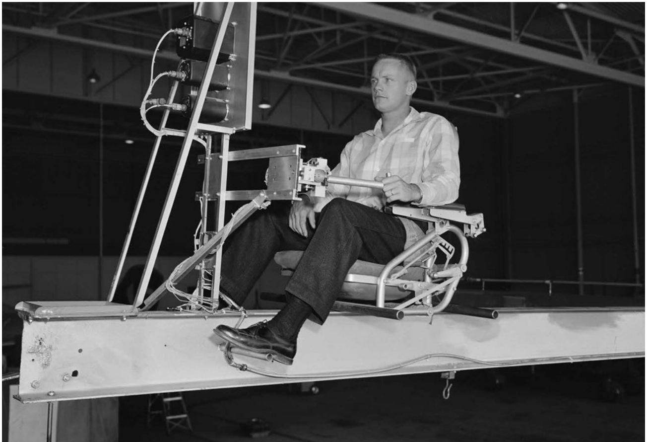
Neil Armstrong at the controls of the Iron Cross. Between the somewhat violent strikes of the I-beams on the hangar floor and motion of the Iron Cross—given the moment arm—the pilots wore seat belts. The controller was mounted horizontally from the instrument panel, as it would be in the X-1B. NASA E56-2607
