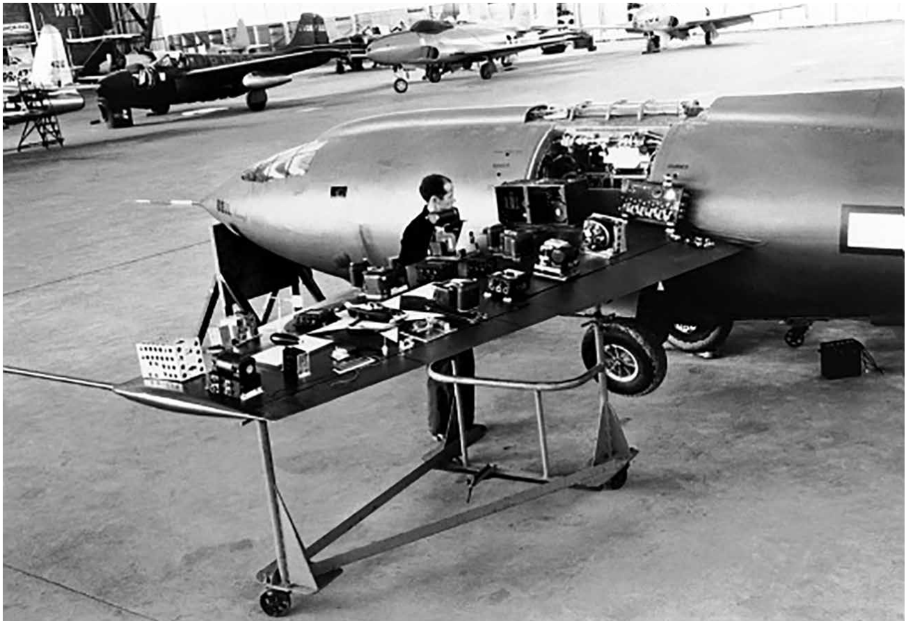
An NACA technician standing in front of the instrumentation the Bell X-1 carried on research flights. NASA E-4837
